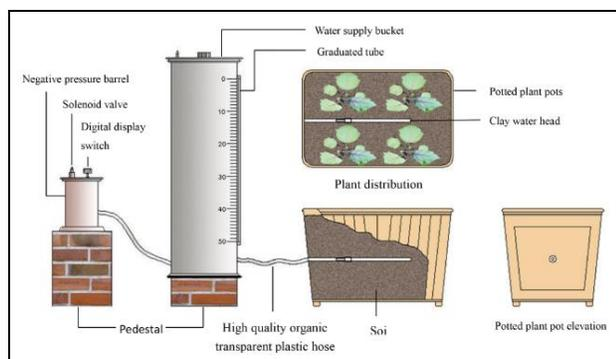
**Fig. 1:** Sketch of stable negative pressure irrigation control device used in this study
